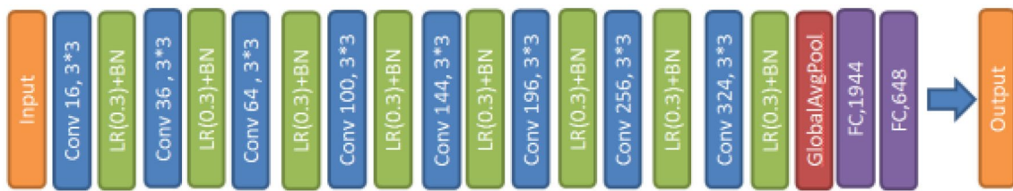
Fig. 7 Architecture of cascade approach for the detection of cystic fibrosis [128]
