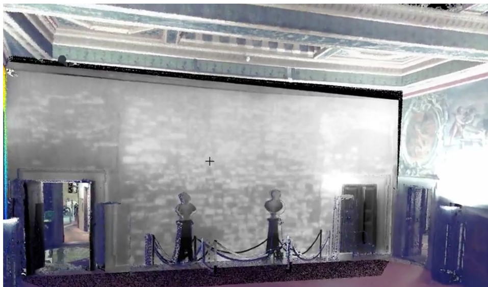
Fig. 5 Example of thermal image mosaic draped onto 3D laser scan model in the Room of the Elements
