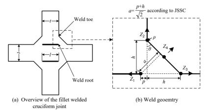
**Figure 4** Weld geometry parameters in a fillet welded cruciform joint (weld toe radius  $\rho$ , flank angle  $\theta$ , slit length *l*, weld leg length *h*, weld penetration depth *p*, weld throat thickness *a*)
