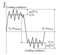
Figure 1 LCF loading for ship structures (Dong et al. 2021b)
