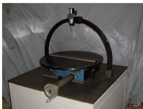
(a) Turn table device with the arc-shape rail dial gauge
