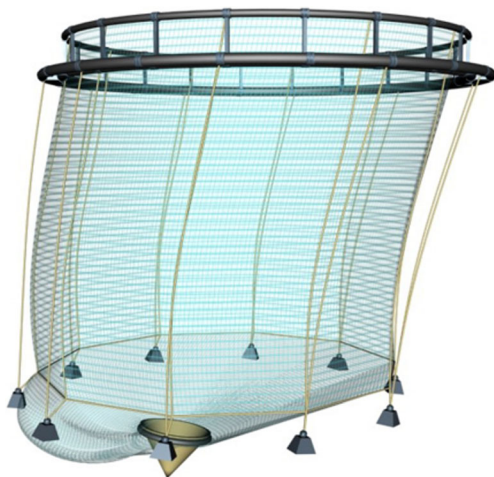
Fig. 1 Floating fish farm with circular plastic collar consisting of two tori that are nearly semisubmerged in calm water, railing, jump net, netting, dead fish removal system, frame of ropes, and bottom weights (Sintef Fisheries and Aquaculture)
