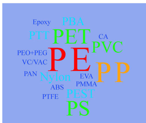
Fig. 2 Word-cloud of the major detected MP materials in raw waters to DWTPs. (Font sizes are determined by the frequencies of detection of the materials in all the studies. For example, PE was reported in all the seven studies on full-scale DWTPs, so PE's frequency is 7. Colors are only for aesthetics. The image was generated using WordItOut at https://worditout.com ).
