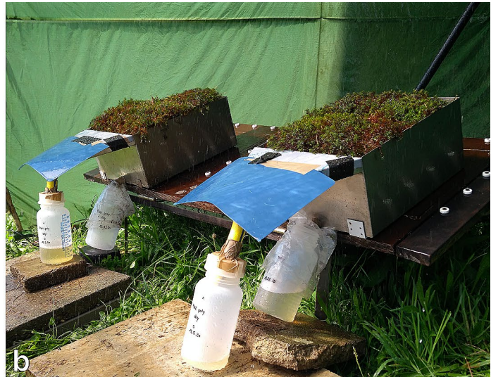
Fig. 2 Illustration of an infiltration box. (a) Technical drawing of an infiltration box (Illustration: Julia Dartsch). (b) Infiltration boxes during rainfall simulations
