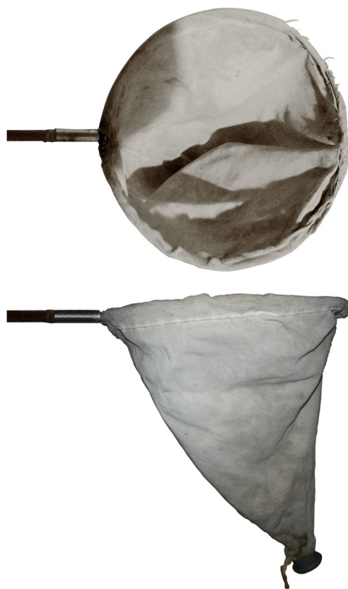
Fig. 2 Sweep net with PVC pipe section to which a transparent double nylon bag for the insect sample is attached (Photo: A. Harris)
