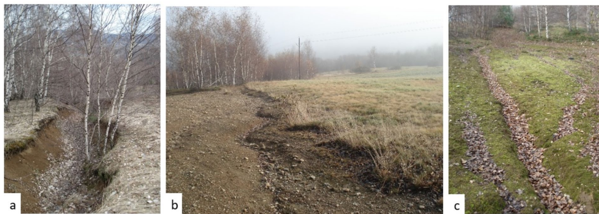
Fig. 1 Artificially created channel for the AMD drainage (a), AMD flowing down the slope, which divided the area into an area heavily damaged by acidification (no vegetation) and a less damaged area
