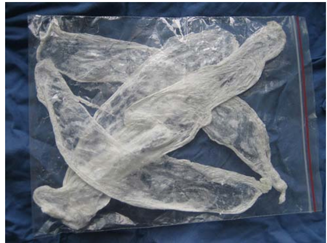
Fig. 3 Macroscopical view of scaffold (SIS straps sealed in a sterile plastic bag). Manufactured SIS is a white membrane-like biomaterial, 100 \pm 20 \mu\text{m} in thickness, and the texture is just as flexible as natural bone membrane. This biomaterial was also easy to handle for clipping, sterile radiation and sealing preservation
