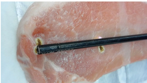
Fig. 1 Forceps with insulation failure and energizing at a location other than the tip (arrow)
