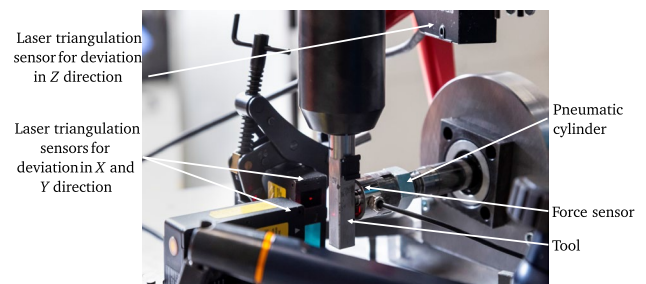
Fig. 3 Experimental setup containing laser sensors and the pneumatic cylinder
