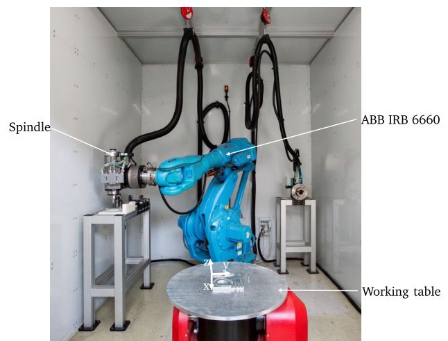
Fig. 2 Robot cell including the ABB IRB 6660-205/1.9 and the effectors
