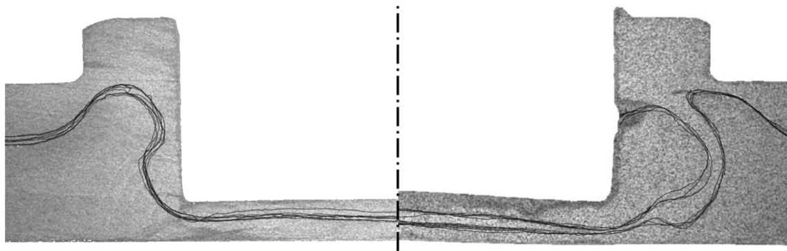
Fig. 3 Separation lines of the conventional flat-clinch joint (left), and the flat-clinch joint with AJE (right)
