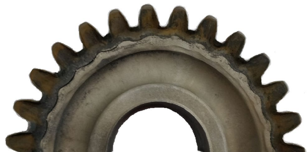
Fig. 4 Forged bi-metal gear from an aluminium centre and exterior steel ring [120]
