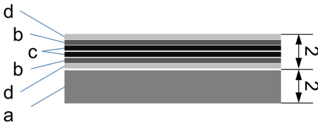
Fig. 2 Layup of the hybrid plate with a steel HC340LA, b Style 423-1, 6K carbon fabric, c 650SA4, 12K carbon fabric and d microlith ST 3022 glass fabric
