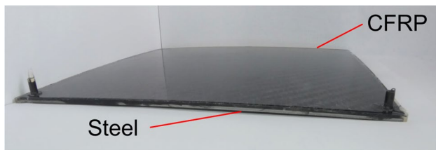
Fig. 4 Picture of a hybrid steel-CFRP plate manufactured with Set #1
