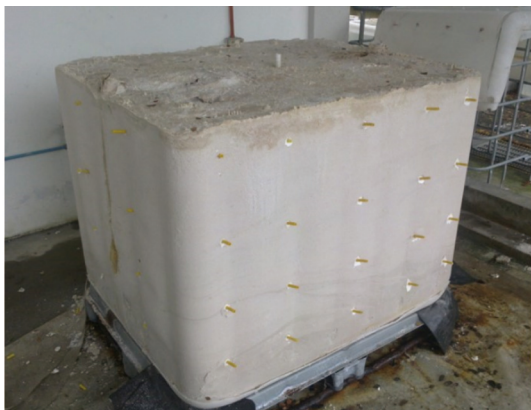
Fig. 5 Up-scaled model tests: 1 m 3 sand model of Wu et al. [293].
