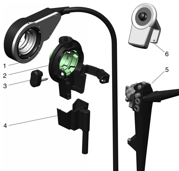
Fig. 2 Exploded view of the add-on platform: 1 remote drive unit, 2 connection module, 3 plug, 4 docking station, 5 endoscope and joystick controller
