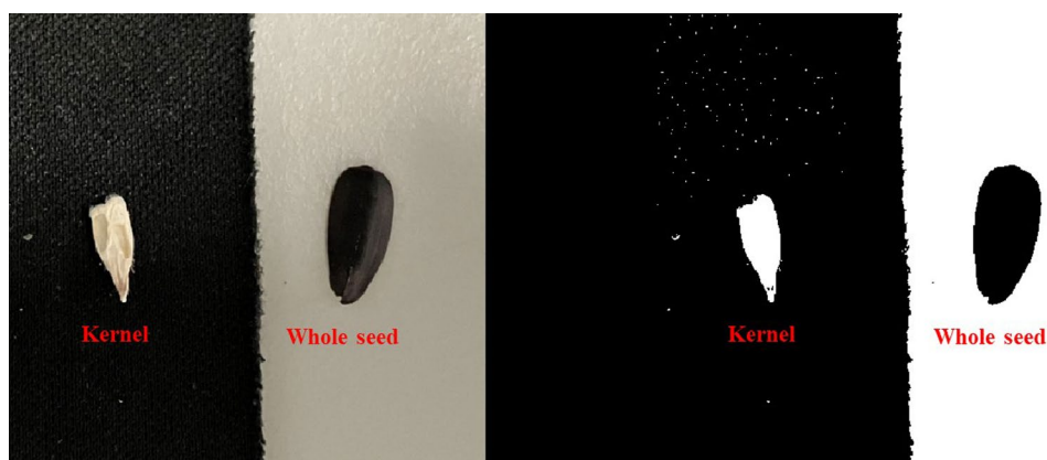
Fig. 9 Image segmentation of kernel and seed for calculating 2D plumpness
