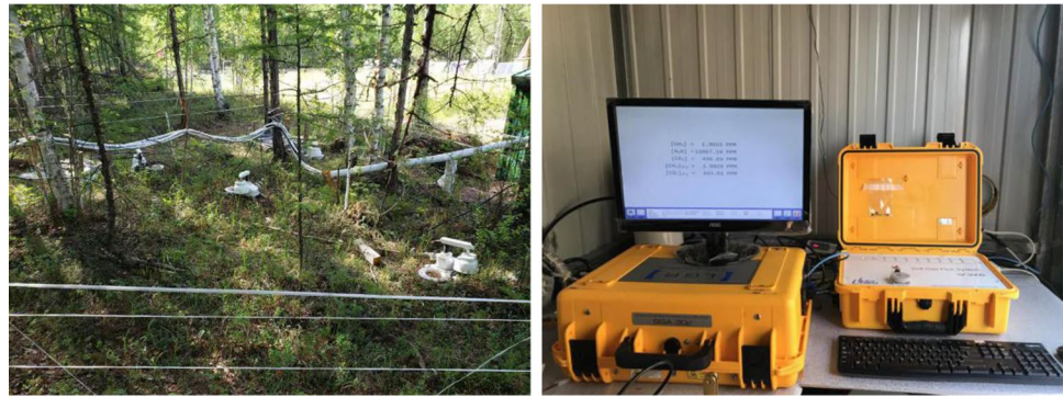
Fig. 2 LGR automatic multi-channel soil fluxes measurement system used in this study during the period of 1 April to 30 September, 2019
