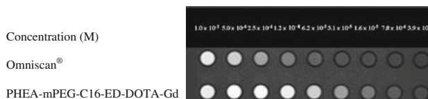
Fig. 4 T1-weighted MR phantom image of PHEA-mPEG-C 16 -ED-DOTA-Gd and Omniscan ®
