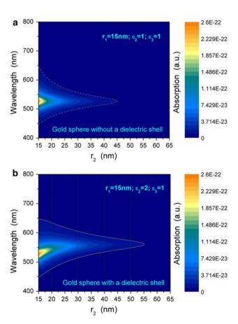
**Fig. 6** Absorption cross-section as a function of wavelength and distance from the gold particle center,  $\mathbf{a} \ \varepsilon_2 = \varepsilon_3$ ,  $\mathbf{b} \ \varepsilon_2 > \varepsilon_3$
