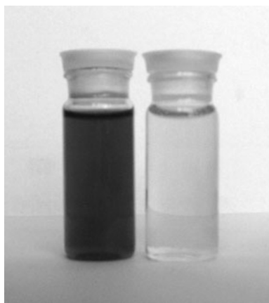
Fig. 3 The color contrast of 100 mg/L MB solution before and after adsorption. The left shows the primary solution, and the right is the solution after adsorption by the porous TiO 2 sample for 10 s
