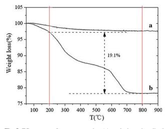
Fig. 5 TG curves of pure magnetite (a) and the mineralized magnetite nanoparticles (b)
