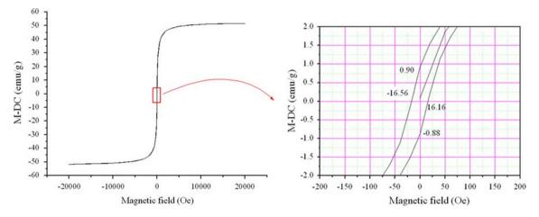
Fig. 6 Hysteresis loop of the mineralized magnetite nanoparticles at 300 K
