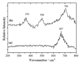
Fig. 3 The Raman spectra of mineralized magnetite nanoparticles (a) and  $\gamma$ -Fe<sub>2</sub>O<sub>3</sub> (b)
