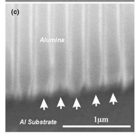
**Fig. 1** ESEM images of a template before and after the complete removal of the oxide barrier layer from the pore bottom tips. **a** Cross-section of an AAO film before the removal of alumina barrier layer; **b** Magnified view of the area marked in **a** with a *white rectangle*; **c** Pore bottom detail on which we can see how the pore bottoms are opened as a whole after the process described has been carried out (the *white arrowheads* indicate the pore bottom tips)
