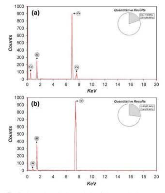
**Fig. 5** Elemental qualitative analysis of the samples by energy dispersive X-ray spectroscopy (EDXS). **a** Spectrum and weight percentage (*inset*) of the elements of the sample corresponding to Co nanopillars; **b** Spectrum and weight percentage (*inset*) of the elements of the sample corresponding to Ni nanopillars
