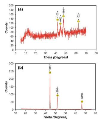
Fig. 6 XRD patterns of cobalt (a) and nickel (b) nanopillar arrays
