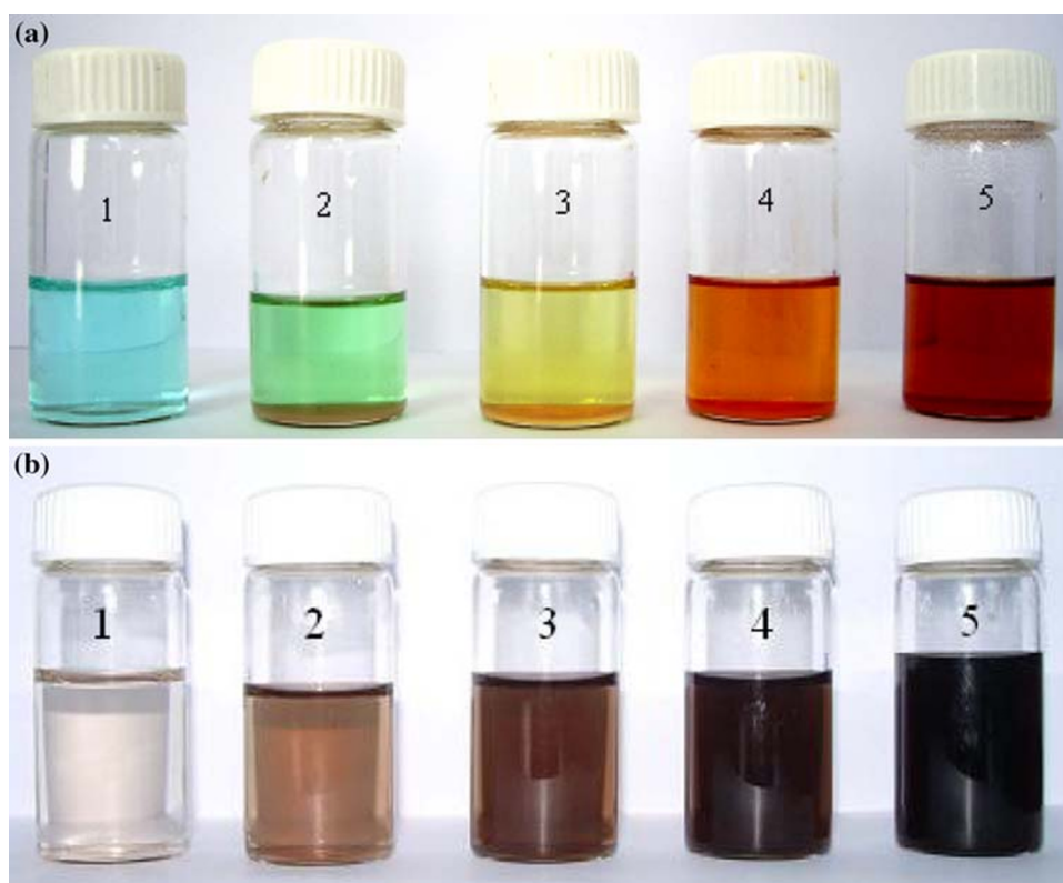
Fig. 1 The color change of the reaction process in water medium (a) and E.G medium (b)
