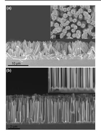
Fig. 1 Cross-sectional FE-SEM images of ZnO nanorods synthesized on the ZnO films prepared by RF sputtering (a) and PLD (b), respectively. The inset in (a) shows the top view of the corresponding sample, the inset in (b) is the corresponding enlarged image
