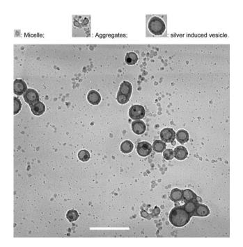
Fig. 1 Formation of nanostructured micelles, aggregates and vesicles in the mixture of cubic and hexagonal phases of  $EO_{20}PO_{70}EO_{20}$  induced by silver nanoparticles. TEM micrograph of vesicles and their ensembles was taken at 200 kV (accelerating voltage). Scale bar: 200 nm
