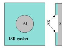
Fig. 6 Spin-coated and photolithographic patterned JSR gasket
