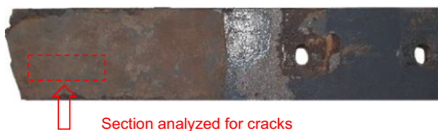
Fig. 25 Place of removal of samples to search for cracks
