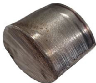
Fig. 6 The shaft end was removed for chemical composition, hardness, and wear analysis
