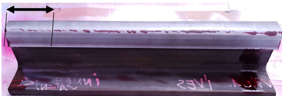
Fig. 4 Evaluation of the ECT, gray–channel 3, black–channel 4
