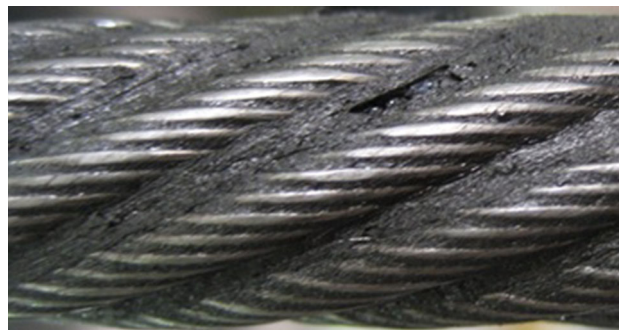
Fig. 11 Lang lay rope. Extracted from KSC-PT technical documentation [5]. Reprinted with permission
