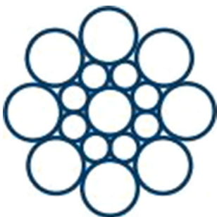
Fig. 7 Non-compacted steel wire rope [13]. Reprinted with permission
