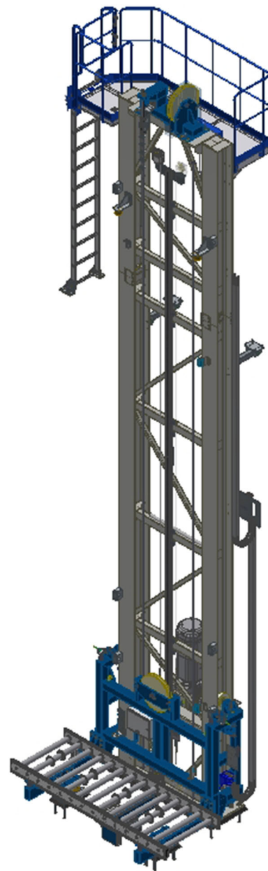
Fig. 2 VTD definition. Steel wire rope VTD designed by the document author for KSC-PT
