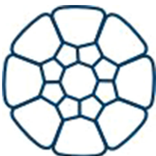
Fig. 8 Compacted steel wire rope [13]. Reprinted with permission
