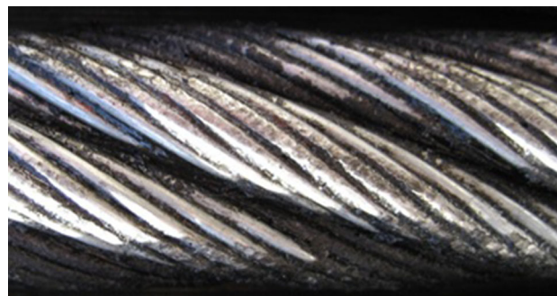
Fig. 12 Regular lay rope. Extracted from KSC-PT technical documentation [5]. Reprinted with permission
