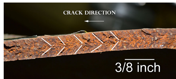
Fig. 6 V-shaped chevron marks found on a pressure vessel brittle fracture surface indicating the direction of crack propagation
