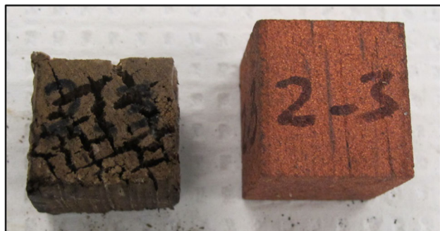
Figure 14 Bare wood (left) and Cu-coated (right) samples after 12 weeks of decay test [47]
