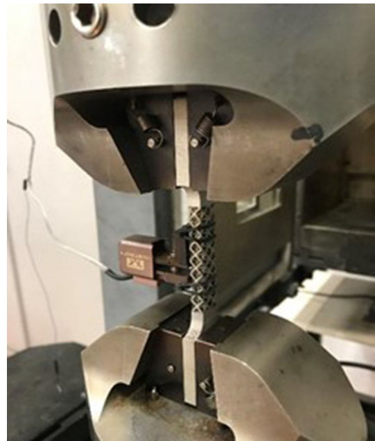
Fig. 3. Experimental setup of the uniaxial tensile test
