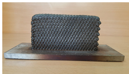
Fig. 1 An example of a WAAM sample fabricated using S355JR steel baseplate
