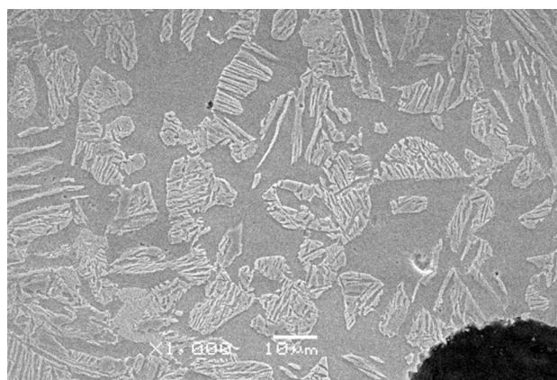
Fig. 7 Microstructure of quenched ductile iron using variant I ( t_\gamma = 860 °C, t_{pi} = 400 °C, \tau_{pi} = 64 ). \times 1000 magnification, SEM, etched using 2% alcoholic solution of \text{HNO}_3
