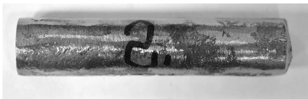
Fig. 1 Macrograph of Co-based alloy cast used in investigation
