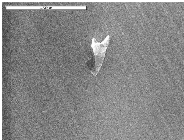
Fig. 4 SEM image of a Ni-graphene coating. Sample 3. Graphene particle in nickel coating
