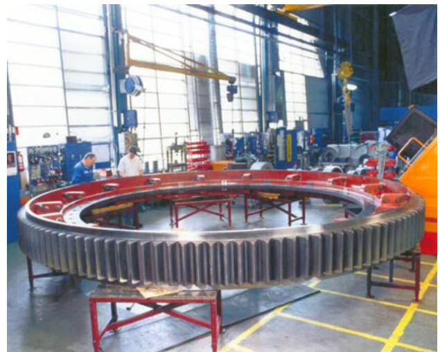
Fig. 18 ADI mill gears are produced in segments and assembled post heat treatment
