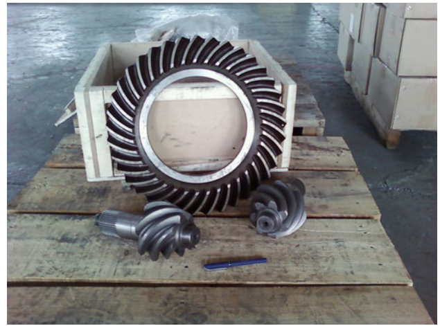
Fig. 16 ADI hypoid differential gears and pinions are common conversions to Grades 1200-850-04 or 1400-1100-02 ADI
