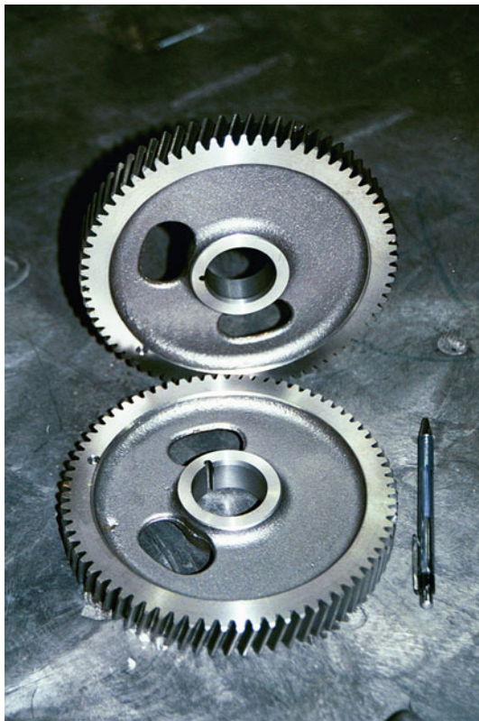
Fig. 15 ADI Diesel engine timing gears have replaced carburized Q&T gears at a cost savings for many years
