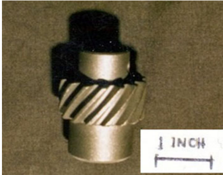
Fig. 20 AGI gear for timing on a light vehicle engine
