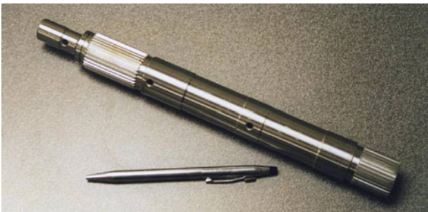
Fig. 28 A Carbo-Austempered™ steel school bus transmission output shaft
