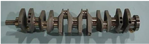
Fig. 19 ADI crankshafts have been used in several notable sports cars for increased fatigue strength and reduced weight and cost (Ref 7)
