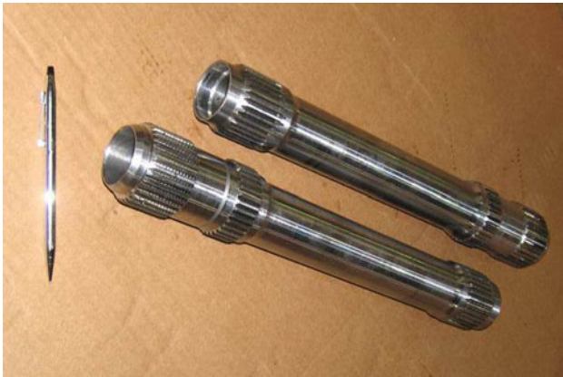
Fig. 23 Austempered steel agricultural transmission output shafts
