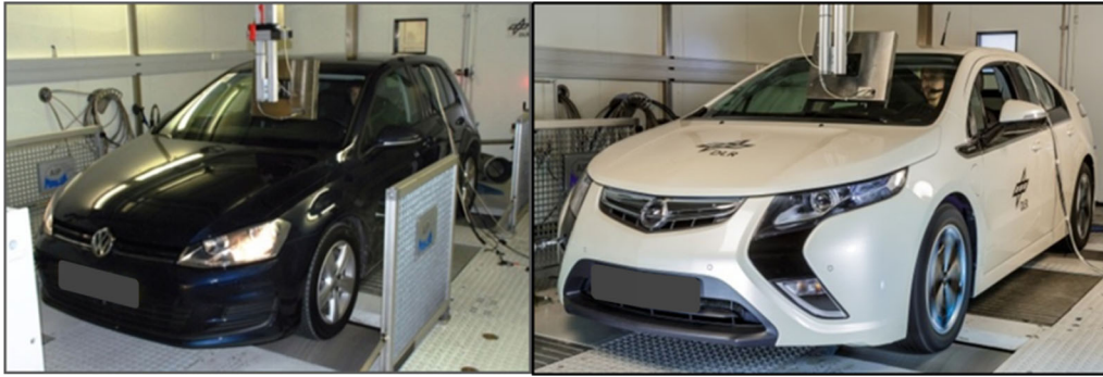
Fig. 2. Reference vehicles at the roller dynamometer test bench.
