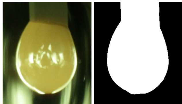
Fig. 3—(Left) Image of a molten \text{Sc}_2\text{O}_3 droplet in the floating zone furnace. (Right) Image processed using Mathematica to produce an outline of the droplet surface.
