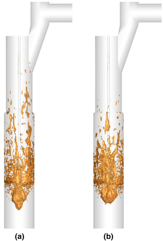
Fig. 5—Two instantaneous snapshots of slag-gas interface for (a) the no-swirl and (b) the swirl configurations.
