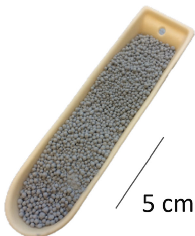
Fig. 1—The 1.25 to 3 mm SiO 2 and SiC pellets after sintering.
