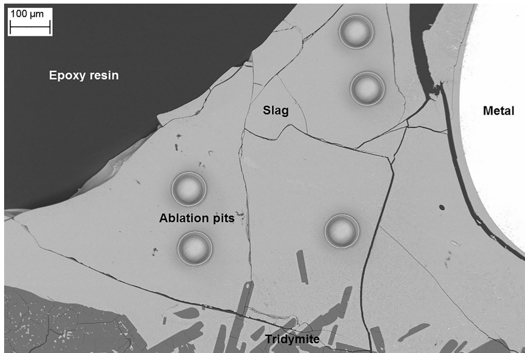
Fig. 2—Ablation pits formed in the glassy slag phase during LA-ICP-MS analysis; a SEM backscattered electron image.
