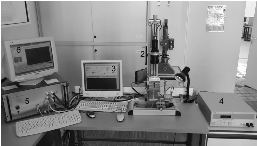
Fig. 2—Setup of the DHTT-equipment: (1) furnace with heating device, (2) height-adjustable stand with camera and objective, (3) temperature control PC monitor, (4) control unit for the furnace, (5) control unit for the heating device, and (6) PC for data storage and visualization.
