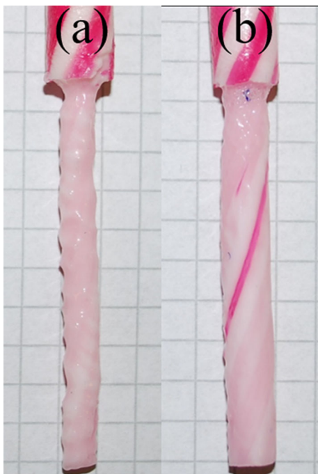
Fig. 7—Photograph of sugar rod (a) in the baffled container and (b) in the cylindrical container after rotating in water at the speed of 100 rpm for 15 min.
