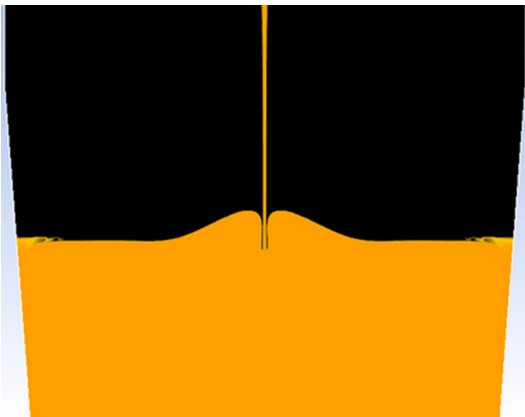
Fig. 2—CFD simulation of plunging tapping jet.
