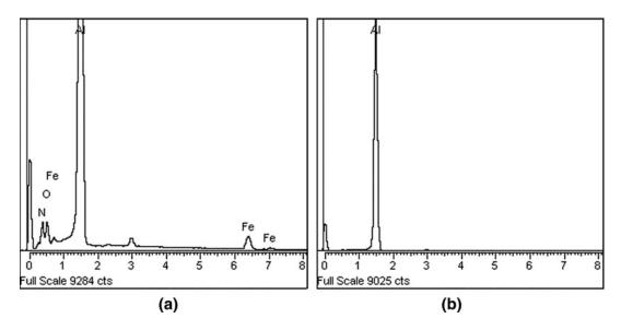
Fig. 16—EDX spectra obtained from points (a) P1 (70.7 Al, 9.5 O, 16.8 N, and 3 Fe) and (b) P2 (100 Al) given in Fig. 15. All concentrations are in weight percent.
