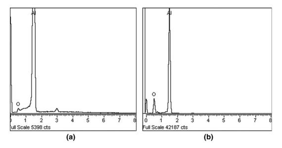
Fig. 5-EDX spectra obtained from points (a) P1 (3.2 wt pct O) and (b) P2 (38.6 wt pct O) given in Fig. 4.
