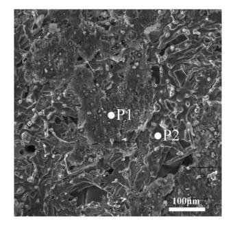
Fig. 15—SEM micrograph obtained from the white area on Fig. 14. The EDX spectra obtained from points P1 and P2 are shown in Fig. 16.
