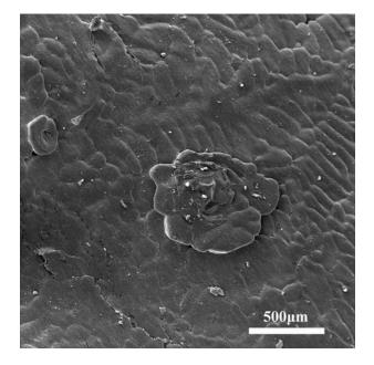
Fig. 6—SEM micrograph of the surface of the oxide layer that was held in the melt for 8 min. The liquid metal exuded from the discontinuity that formed on the layer.
