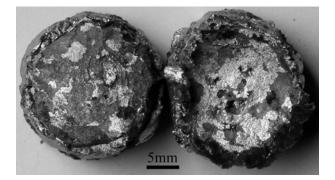
Fig. 18—Photograph of the oxide layers that were held in the liquid metal for 48 h.
