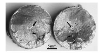
Fig. 2—Photograph of the oxide layers that were held in the liquid metal for 8 min. Two locations in which the oxide layers were bonded to one another are shown by arrows.
