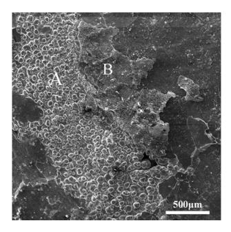
Fig. 10—SEM micrograph of the surface of the oxide layer that was held in the melt for 5 h, showing that the oxide layer was peeled off in area denoted A, and a part of the opposite oxide layer bonded to this oxide surface.
