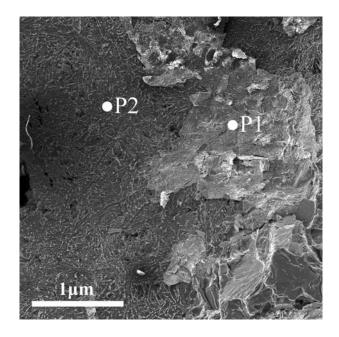
Fig. 21—SEM micrograph obtained from the surface of the oxide layer that was held in the melt for 48 h, showing a microstructure similar to that observed in Fig. 15. The concentration of elements was determined by EDX to be 64 wt pct Al, 12.2 wt pct O, 18.9 wt pct N and 4.8 wt pct Fe on point P1, and 100 wt pct Al on point P2.
