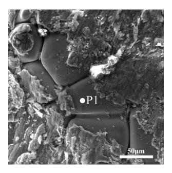
Fig. 12—SEM micrograph of the surface of the oxide layer that was held in the melt for 5 h, showing a crack that formed on the oxide layer, perhaps during the solidification of the specimen. The EDX spectra obtained from point P1 is shown in Fig. 13.
