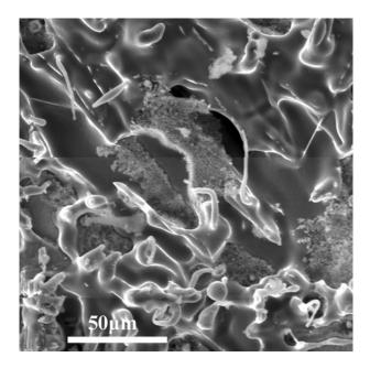
Fig. 17—Another SEM micrograph showing the AlN phase on the Al dendrites, taken from the oxide layer that was held in the melt for 16 h.
