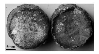
Fig. 14—Photograph of the oxide layers that were held in the liquid metal for 16 h, showing vast white areas on one side, which matched with vast darker areas on the other side.
