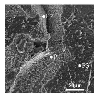
Fig. 19—SEM micrograph of the surface of the oxide layer that was held in the melt for 48 h, showing an oxide layer over an AlN layer. The EDX spectra obtained from points P1 to P3 on this figure are shown in Fig. 20.
