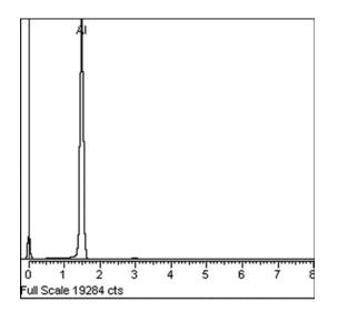
Fig. 13—EDX spectrum obtained from the point denoted P1 on Fig. 12. The absence of O peak in this spectrum confirmed that the O was not present in the trapped atmosphere of the defect at the holding time of 5 h.
