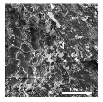
Fig. 11—SEM micrograph of the surface of the oxide layer that was held in the melt for 5 h, showing that the oxide layer was peeled off from the surface of the oxide.
