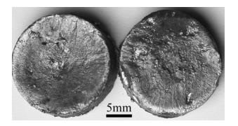
Fig. 7—Photograph of the oxide layers that were held in the liquid metal for 1 h.
