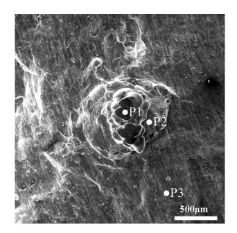
Fig. 8—SEM micrograph of the surface of the oxide layer that was held in the melt for 1 h. The concentration of O was determined by EDX to be 8.4, 49.4, and 21.6 wt pct on points P1, P2 and P3, respectively.
