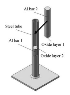
Fig. 1—Schematic illustration of the steel tube and the two inserted Al bars. After melting, the oxide layers 1 and 2 and the atmosphere trapped between them represented a double-oxide film defect in a liquid Al alloy.
