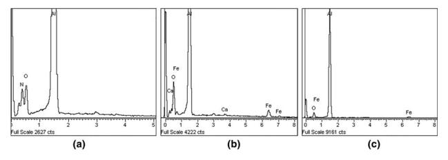
Fig. 20—EDX spectra obtained from points (a) P1 (65.7 Al, 15.9 O, and 18.5 N), (b) P2 (75.3 Al, 21.4 O, and 3.9 Fe), and (c) P3 (75.2 Al, 20.5 O, and 4.3 Fe) given in Fig. 19. All concentrations are in weight percent.
