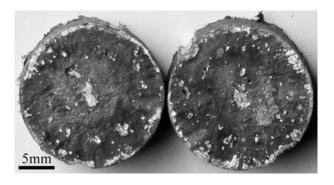
Fig. 9—Photograph of the oxide layers that were held in the liquid metal for 5 h. The number of points bonded to one another increased considerably compared with the previous specimens.
