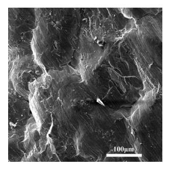
Fig. 3—SEM micrograph of the surface of the oxide layer that was held in the melt for 8 min. Some discontinuities in the oxide layer are visible. A higher magnification micrograph of this oxide is shown in Fig. 4.
