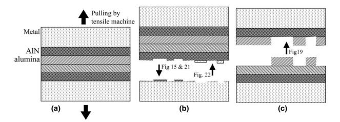
Fig. 23—Schematic illustration of the ways that the two Al bars detached from one another during the separation of the Al bars by the tensile test machine. (a) Before the separation of the Al bars. (b) The AlN layer was separated from the metal. (c) The two oxide layers did not bond to one another in some parts; however, the alumina layer was detached from the AlN layer in the areas that the two oxide layer did bond.
