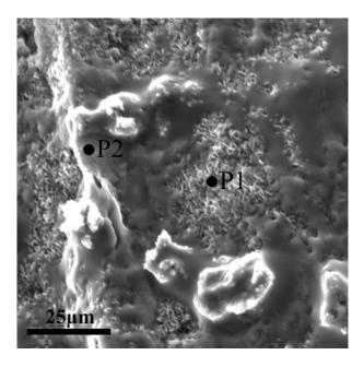
Fig. 22—Another SEM micrograph obtained from the surface of the oxide layer that was held in the melt for 48 h, showing Al dendrites remaining on the AlN layer when the two Al bars were pulled apart by the tensile machine. The concentration of elements was determined by EDX to be 70.2 wt pct Al, 8.3 wt pct O, 20.6 wt pct N and 0.9 wt pct Fe on point P1, and 100 wt pct Al on point P2.
