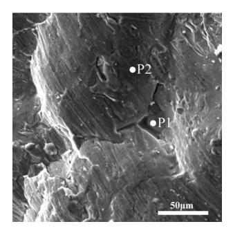
Fig. 4—A higher magnification SEM micrograph of the oxide layer shown in Fig. 2. The EDX spectra obtained from points P1 and P2 are shown in Fig. 5.
