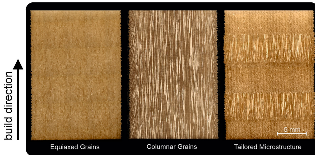
Fig. 5—Typical EBM Alloy 247 grain microstructures within specimens of \varnothing 15 mm. The process parameters are defining melt pool shape, solidification velocity and temperature gradients and control whether a poly crystalline and equiaxed (left) or a highly anisotropic columnar (center) grain microstructure is remaining in the specimens. Local tailoring of the microstructure was possible as-well and demonstrated by alternating PS and DS in certain z-heights (right).
