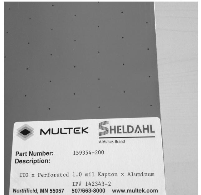
Fig. 1—A picture of a foil that was used in our experiments and its specification.
